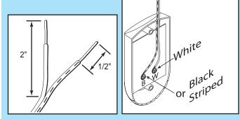
FIG. 3-2 Splitting and stripping.
